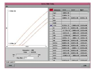
Slider view enables interactive curve-fitting of the model to the data, providing insight into the sensitivity of the model to a particular parameter.
