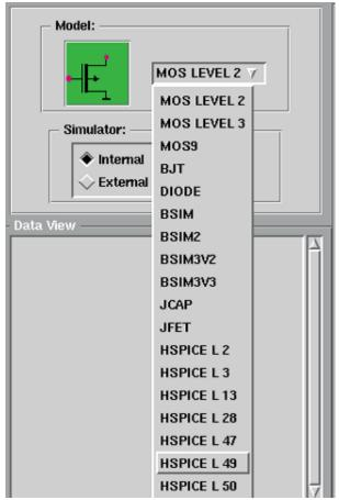
The list of built-in models available in Aurora facilitates extraction of parameters for UC Berkele well as Star-HSPICE implementation of the models
