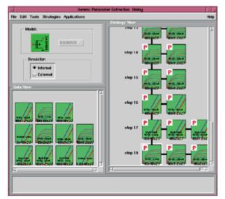
The main aurora window represents data files and strategy steps as icons. To create strategy s data icons are dragged and dropped with the mouse from the Data View section to the Strategy View section. The ranges of variables, targets, and optimizable parameters are then specified.
