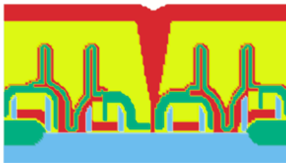
Figure 4d: 2D cross-sectional view showing misalignment
